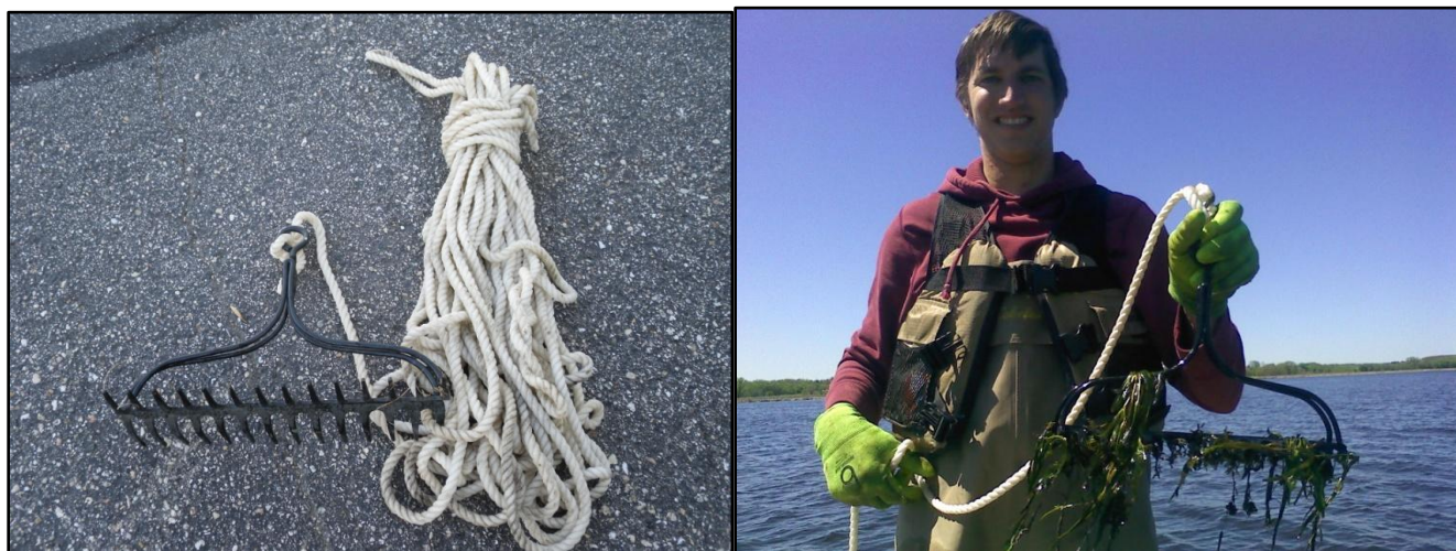
Figures 1 and 2. Double-headed, weighted garden rake, attached to a rope used to survey aquatic vegetation.
